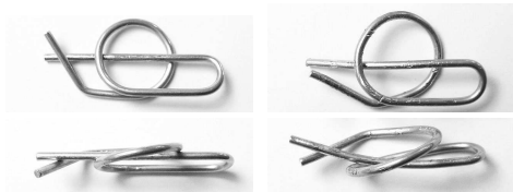
Ring cotter o.k. Change the ring cotter Fig. 15: Condition of the Rue ring cotter [1a]
