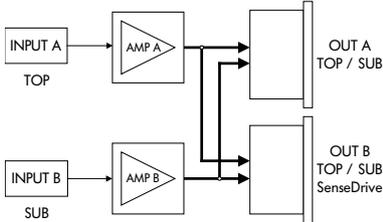
**D12 Input/Output routing
