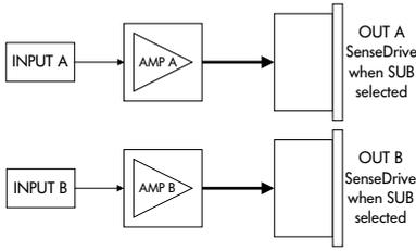
**D12 Input/Output Routing
