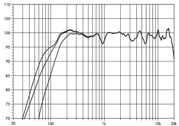
**MAX12 frequency response (linear setup, free field) CPL +5, standard and CUT**
