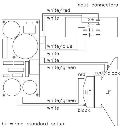
bi-wiring standard setup
