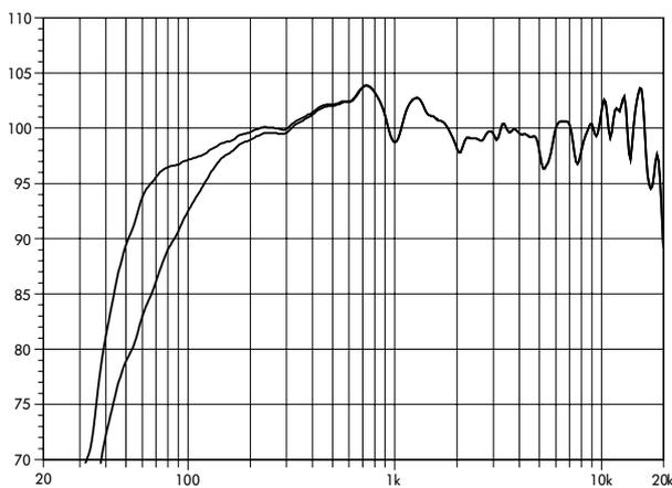
**MAX12 frequency response (MAX setup, floor coupling), standard and CUT**
