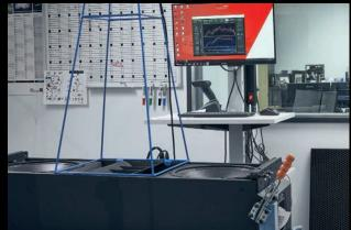
Finally, the functionality of all technical components, such as drivers and crossovers, are tested according to original specifications as for new goods and replaced if necessary.
