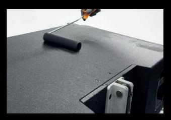
...and completely repainted with the original d&b topcoat.
