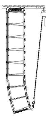
Compressed array with motorized chain hoist
