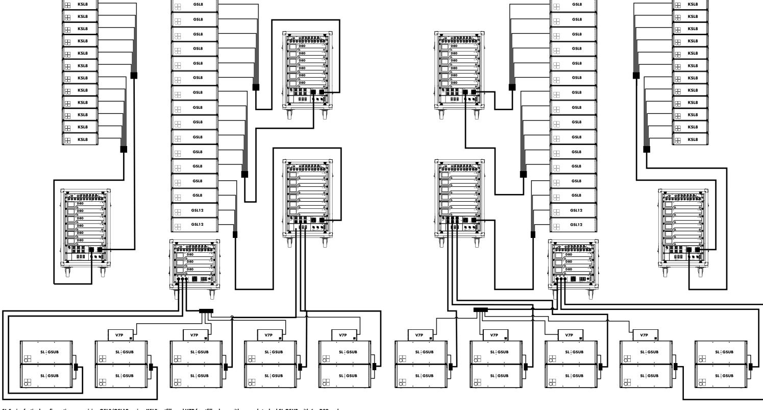
SL-Series festival configuration comprising GSL8/GSL12 mains, KSL8 outfills and V7P frontfills along with ground stacked SL-GSUB with 6 x D80 and 3 x D80 Touring racks
