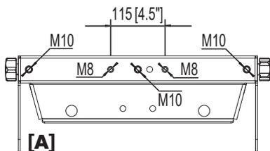
**Fig. 4: Threaded inserts of the outer bracket [A]**
