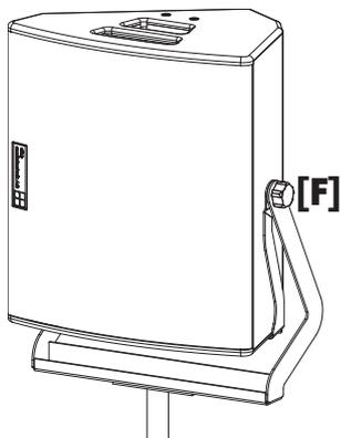
**Fig. 6: Z5056 M4 Flying bracket operation**
