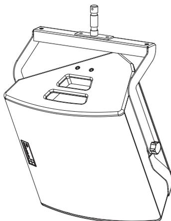
**Fig. 7: Z5056 M4 Flying bracket with Z5010 TV spigot**
