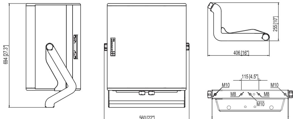
**Fig. 2: Z5056 M4 Flying bracket dimensions in mm [inch]**
