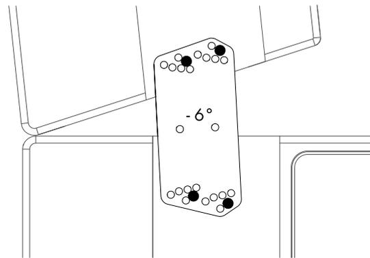
**Fig. 4: Z5421 Connector plate xA, neg. splay, angle setting**
