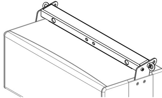
**Option 3:** Suspension of the array using the Z5419 Load bar xA together with 2 x 1t shackle, e.g. d&b E6507.
