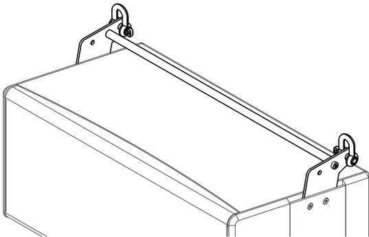
**Option 4:** Suspension of the array using the Z5419 Load bar xA together with 2 x Z5420 Load eye bolt.
