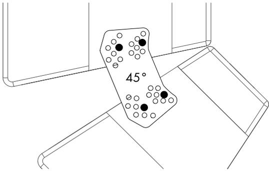
**Fig. 1: Z5416 Connector plate 10A, angle setting**
