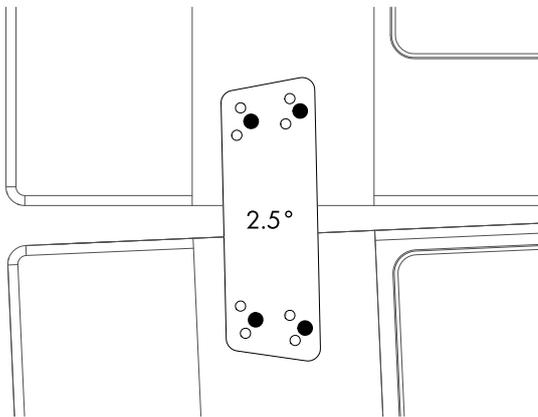
**Fig. 3: Z5418 Connector plate xA-SUB, angle setting**
