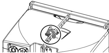
The selected hole position defines the vertical aiming of the entire array using the array's center of gravity.
