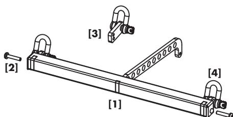
Fig. 1: Z5374 Ti Flying bar components
