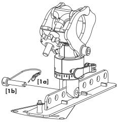
Rota clamp assembly with flying adapter
