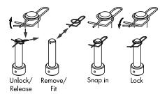
**Fixing bolt secured** Function of the securing pin (ring cotter)
