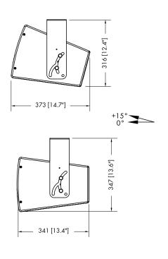
Z5398 Mounting options 1,2 and 3 with built-in dimensions in mm [inch]
