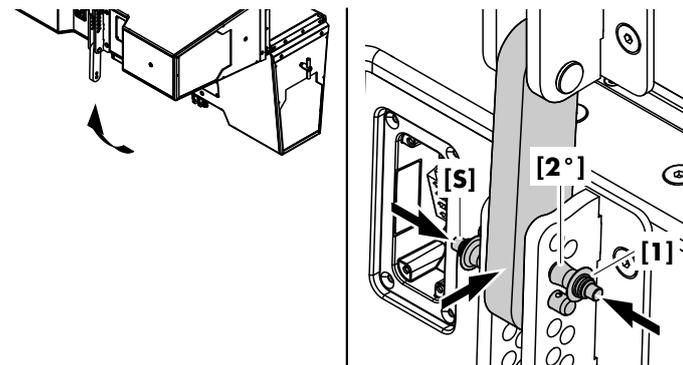
6. Insert and handtighten the fixing bolts of the upper cabinet's Front links on both sides.
