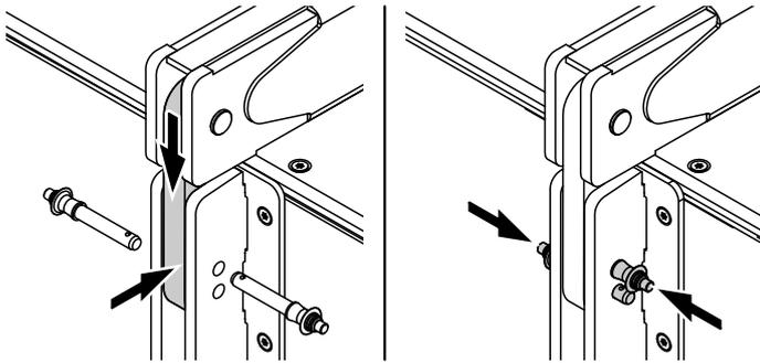
4. At the rear, check the Rear link is properly fitted into the rear rigging strand of the cabinet.
