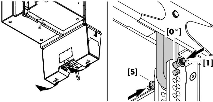
7. Raise the back of the cabinet until the Rear link of the adapter fits into the rear rigging strand of the cabinet.
