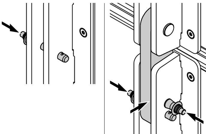
7. At the rear of the upper cabinet, reinsert the Locking pin that holds its Rear link in its park position.
