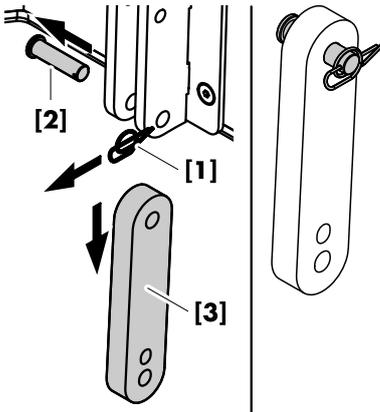
7. Raise the bottom cabinet until the Splay link of the upper cabinet fits into the rear rigging strand of the bottom cabinet.
