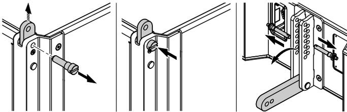
1. Prepare the Front and Splay links of the next cabinet as described in ⇒ Chapter 2.5.1 "Front link mechanism" on page 13 and ⇒ Chapter 2.5.2 "Splay/Rear link mechanism" on page 14.
