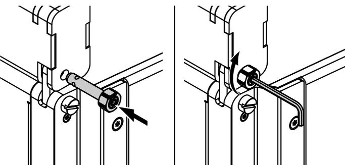
**Type [B]** Locking pin 10 x 45 mm used for the Mounting adapter's Rear link slot.
