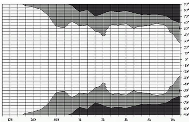
Isobar diagram E12-D horizontal, horizontal setup with the horn rotated
