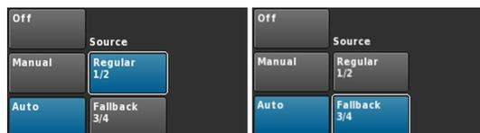
After the Fallback function has been triggered, it can be reset manually by reactivating (selecting) the «Regular 1/2» input source.
