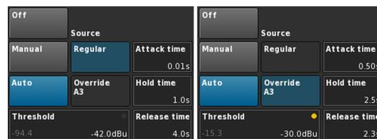
As soon as the signal level drops below the threshold, input A3 will be muted while all other channels will be unmuted depending on the set Hold and Release times (crossfade).
