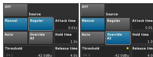
**Auto** With this mode selected, the analog input A3 is permanently monitored. As soon as the incoming signal level exceeds the defined threshold, input A3 will be opened depending on the set Attack time. All other inputs will be muted (Gate + Ducking).
