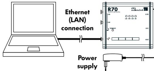
**Note:** When Power over Ethernet (PoE) is available, the external power supply is not required.
