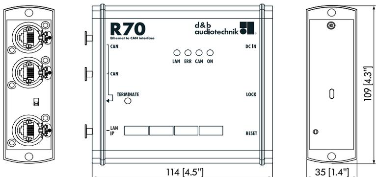
**Fig. 1: Dimensions in mm [inch]**
