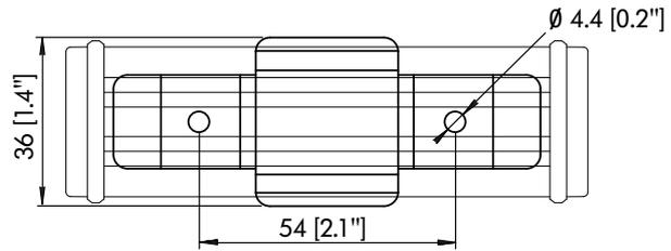
**Fig. 7: Z6123 Bopla mounting clamp upright, dimensions in mm [inch]**
