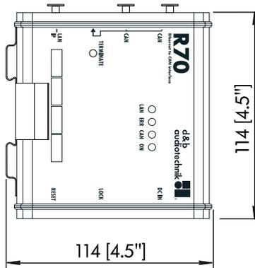
**Fig. 8: Wall mounting with dimensions in mm [inch]**
