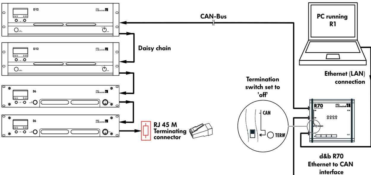
Fig. 6: d&b Remote network (CAN-Bus), wiring example 2 with non-terminated R70 interface within the CAN-Bus segment.
