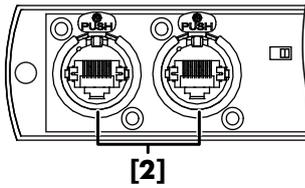
Two RJ 45 connectors are located on the left hand side panel of the device. Both connectors are wired in parallel to allow different wiring setups of the CAN-Bus
