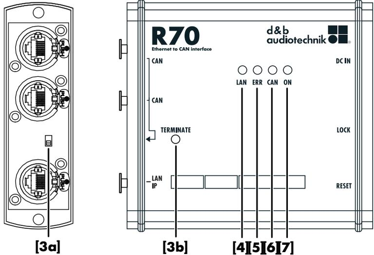
**Fig. 2: Controls and indicators**
