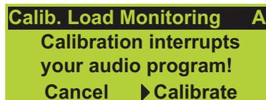
Selecting "Calibrate" starts the calibration procedure while the progress of the procedure is displayed. It can be canceled/interrupted and restarted at any time by pushing the encoder during the procedure.
