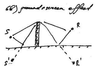
Possible to introduce measured data for special types of barriers
