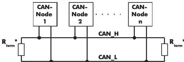
**Fig. 5: Connection of nodes to the bus**
