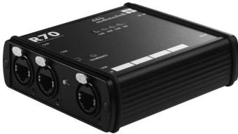
The Z6124 R70 Ethernet to CAN interface provides two RJ 45 CAN connectors with a built-in switchable terminator as well as a LAN connector. The R70 contains a web interface and does not require its own drivers for use with a computer. All configurations can be set using a standard web browser with JavaScript enabled.
