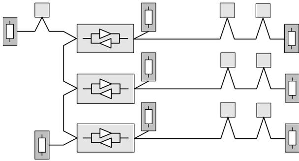
**Fig. 4: Star wiring with repeaters**
