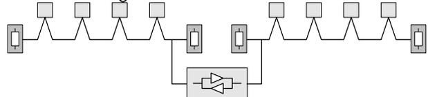
Fig. 3: Connecting two CAN segments with a repeater
