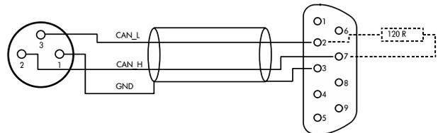
**Fig. 10: XLR to D-SUB 9 F adapter cable**
