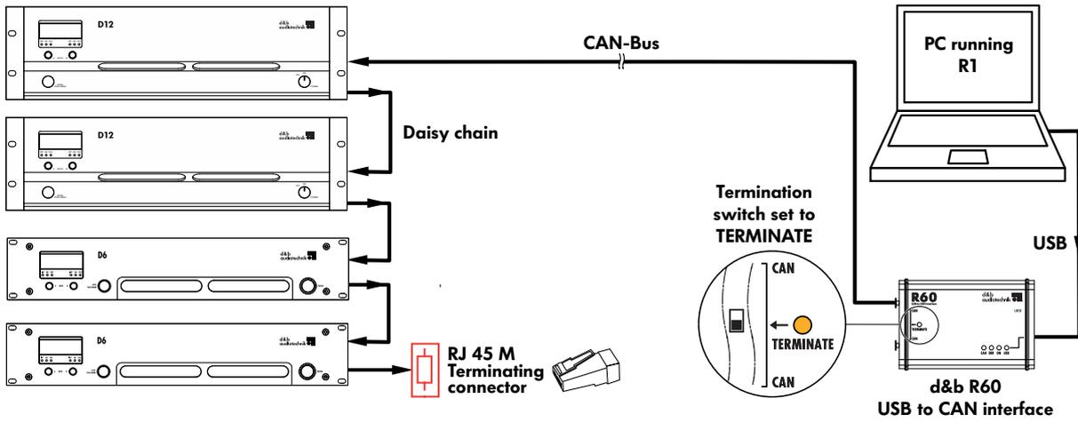
**Example 1: Simple setup with terminated interface at the "beginning" of the CAN-Bus segment.**
