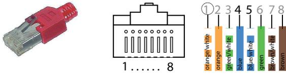
**Fig. 6: RJ 45 connector with metal housing (shield - CAN ground), RJ 45 pin number identification (viewed from the front), and color code according to T568B standard.**
