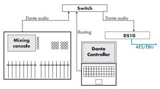
Once all devices are connected, they are detected by Dante Controller and shown in a matrix view with all available inputs and outputs. Audio routings can be set by placing checks at the desired crosspoints within the matrix. Besides device discovery, further configuration settings such as the assignment of IP addresses or clocking also work automatically and do not normally require any user interaction, even in large systems.
