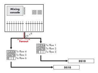
In such cases, the use of **multicast** should be considered. Multicast flows have to be specifically generated in Dante Controller. In contrast to unicast flows, they contain up to eight audio channels and need to be generated only once regardless of the number of subscriptions to these channels. At the transmitter, there is no duplication of traffic or flows, rather switches handle multicast flows by outputting them through all ports, thus flooding the network.
