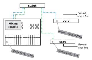
This parameter is vitally important with regard to simultaneous playout from different Dante enabled devices. Considering one DS10 per side driving a large PA system, both of them have to be set to the same latency value. Additionally, in case of a live event, this value should be as low as possible.
