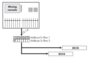
However, due to this flood of data packets further regulatory measures are recommended when multicasts are used in order to prevent the overloading of network segments or devices.
