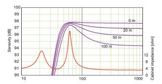
The impedance varies significantly over the low frequency spectrum, in particular with vented or bandpass subwoofer designs. So the effect of the resistance of the cable not only changes the level, but also the tuning and sound character of the system.
