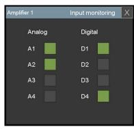
The Input Monitoring screen visualizes the current state of input monitoring for all four analog and digital input channels. The input monitoring states can be changed there as well.
