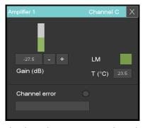
The channel screen contains channel specific controls. In addition to the + and – buttons and display of the current gain in decibel, there's also a slider control to visualize the current gain setting. It can also be used to fade in/out.
