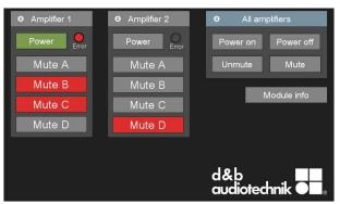
The main screen enables users to change the power and mute states of individual amplifiers and channels. The colors of the buttons provide a visual feedback of the device's power and mute states. Updates from the amplifiers are being processed immediately without timeand resources-consuming polling mechanism for changes in regular time intervals.
